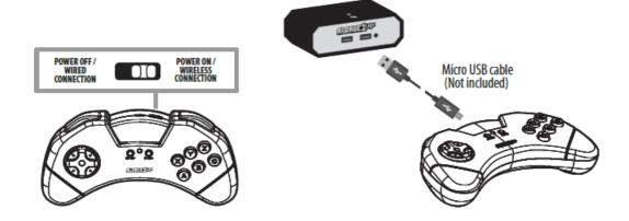
Turn the controller power switch to the left if you use wired connection. Turn to the right if you use wireless connection.
