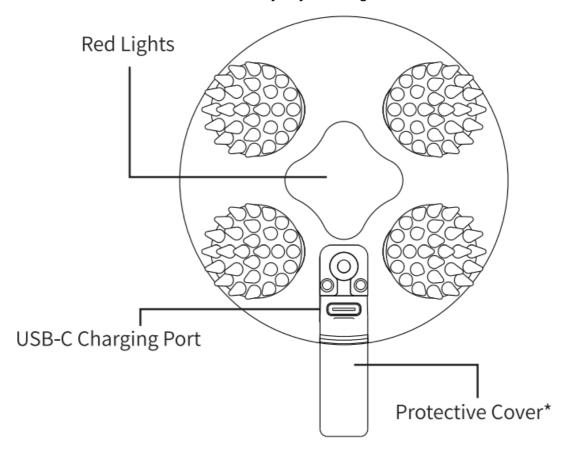
Charging port: two-layer waterproof design, Inner layer access for charging
