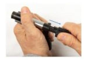
o Using a 9/16 inch or a 14mm wrench, or a crescent wrench, unscrew the breech face from the bolt body.
