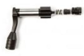
o Reassemble in reverse order. When installing the bolt shroud and firing pin back into the bolt body, align the small tab on the shroud with the corresponding groove in the bolt body. Press the bolt shroud, compressing the firing pin spring, until it can be rotated back into position. When the firing pin clicks into a small detent, just before the angled cut in the bolt, it is correct.
