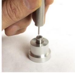
**WARNING:** Attempting to remove an unfired primer in this manner could result in the primer detonating. This could cause injury to eyes from debris and ears from noise.
