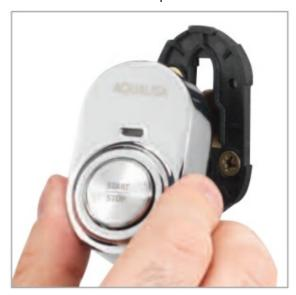
7. Secure the button to the back plate by carefully but firmly pushing the button assembly onto the locking clip at the bottom of the back plate.
