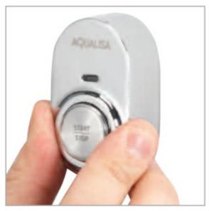
To release the button, insert a small flat bladed screw driver into the small slot at the bottom of the button assembly, to release the locking clip, taking care to avoid damaging the plated surface. Carefully lift the button out and up off of the back plate top locating peg.
