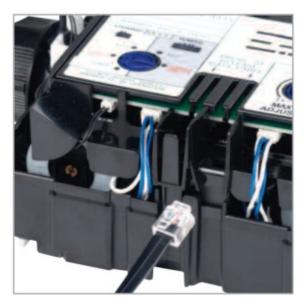
9. Plug the other end of the 2m data cable (supplied with the Digital Diverter) into port 2 on the Digital Diverter.
