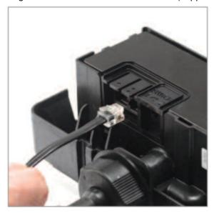
10. Plug the end of the attached data cable feeding from the splitter box into port 1 of the Digital Diverter.
