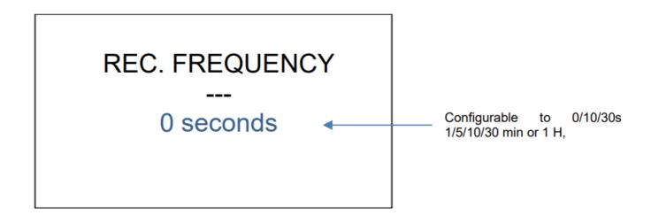
By default, the value is 0 seconds (blue writing), a ONE-OFF recording mode that is triggered by pressing the OK key on the main screen. When recording is enabled on the main screen, the recording icon appears. The frequency can be changed (to 10s/30s, 1/5/10/30 min or 1 H) using the up and down arrow keys (the writing changes to white). Press the OK key to confirm the chosen frequency (writing turns green). To return to the previous menu select the Escape (ESC) key.
