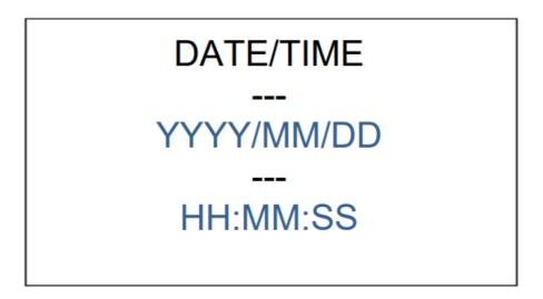
To change the date and time place the cursor on the desired line and use the Up/Down arrows to change the numbers from 0 to 9. The writing then changes to white. Confirm your setting with the OK key (the writing changes to green).
