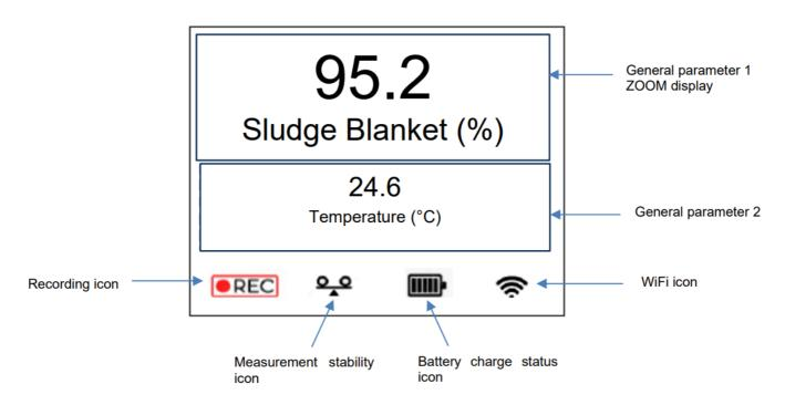
When General parameter 1 changes, there is no measurement stability icon and the measurement fluctuates. When this parameter is stable, the stability icon appears and the measurement flashes.
