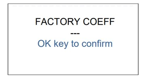
To validate the setting the factory coefficients in the sensor, confirm with the OK key then press Escape (ESC) to return to the previous screen.
