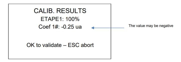
To validate the calibration and complete this procedure, press the OK key. If the calibration is rejected, press the Escape (ESC) key.
