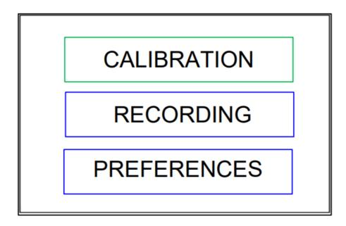
Move the cursor with the up and down arrows to access the desired menu and confirm the selection with the "OK" key. Press the "ESC" key to return to the previous screen.
