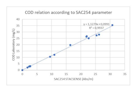
The linear regression line proposes a new relationship between the UV absorption at 254 nm (CAS254) and the CODeq -> CODeq = 1.1279 \* CAS254 + 0.0991.
