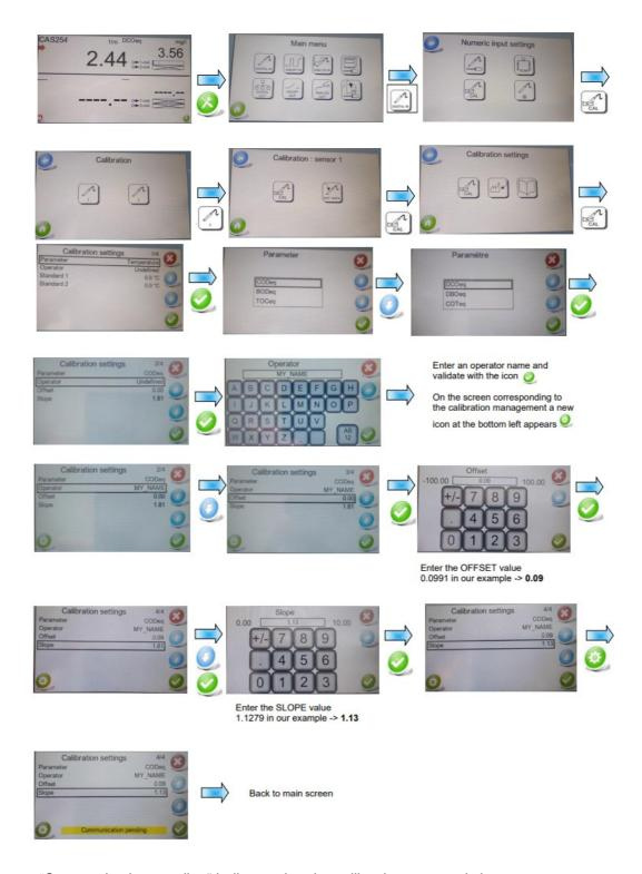
The message "Communication pending" indicates that the calibration process is in progress.
