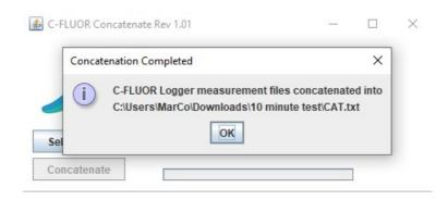
Press 'Concatenate' to begin measurement processing. The software reads all C-FLUOR Logger data files in the DATA Folder. These are written to the same folder. The software presents a dialog window when the process is completed.
