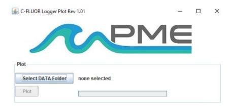
C-FLUOR Concatenate concatenates the files recorded by the C-FLUOR Logger. The software reads all Logger files in a folder, except the CAT.txt file. Software translates Logger timestamps into two additional formats and saves the result in a CAT.txt file in the DATA folder.
