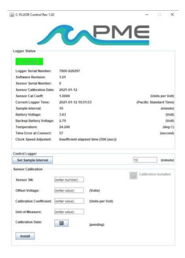
The current Logger sample interval will be displayed next to the Set Sample Interval button. If this interval is acceptable the interval need not be set.
