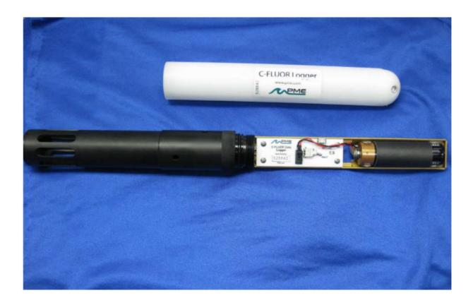
Always install fresh desiccant when closing up the Logger. Moisture buildup can cause issues with the electronics.
