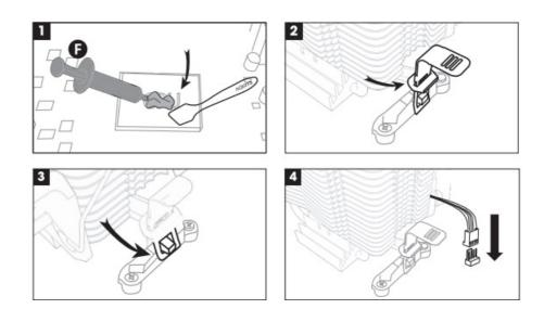
Connect the 4-pin PWM cable of the fan fo the CPU\_FAN connector on the motherboard.
