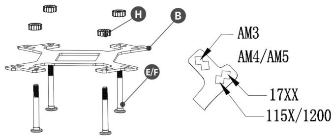
Install the pump and secure it to the backplate using screws (E) For socket I I 5x/I 200 or (F) For socket 1700. Before beginning the pump installation, do not forget to install the spacer (S) and washer (R) to ensure the correct and stable mounting of the pump. Tighten the opposite screws (M) gradually and in turn (diagonally) without applying excessive force at the end.
