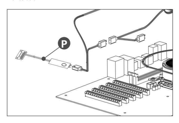
If the motherboard is not ARGB compatible, to activate and control the lighting, the controller (PI included in the package is used. Follow the steps For synchronizing the lighting with the motherboard, but instead, in the end, connect the 3-pin ARGB female connector to the external ARGB controller. Connect the ARGB controller to a free SATA connector from the PC's power supply. The lighting effects are controlled by pressing the button located on the ARGB controller.
