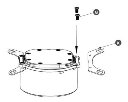
Attach the AMD brackets (K) to the pump using the screws (Gland following the positioning in the image.
