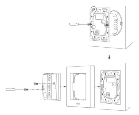
4. Attach the switch plate to the switching unit.
