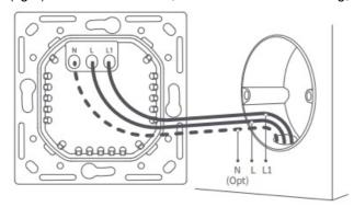
3. Mount the power unit of the switch to the wall junction box with the attached screws and mount the switch frame. Align the pins of the switching unit with the power unit, and snap them together, then use provided screws to securely fasten them in place.
