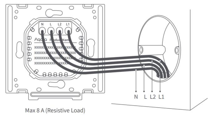
4. Use the included screws to secure the switch to the wall junction box and snap on the panel. Ensure you follow the panel's snap-on installation instructions carefully.
