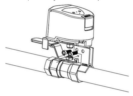
3. Adjust the pipe fixture, turn the screw to loosen the fixture, and thread the fixture through the hole under the bracket to finish installing the bracket and fixture.
