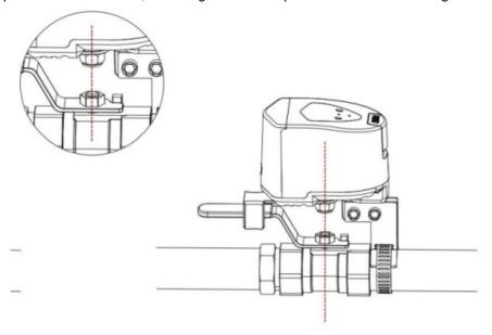
5. Tighten the mounting screws to secure the pipe clamps around the pipe and ensure the equipment's stability.
