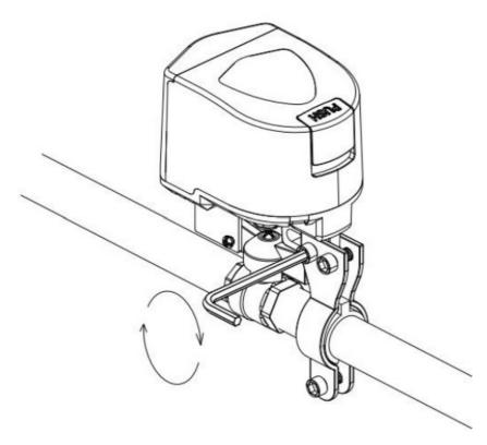
7. According to the style of the butterfly handle, adjust the screws of the clamp to ensure that the fixture can secure the butterfly handle without any interference during operation.
