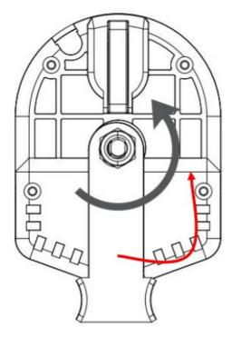
4. Install the butterfly handle swing arm onto the device in the following order: nut from the accessory package, swing arm, and then the securing nut.
