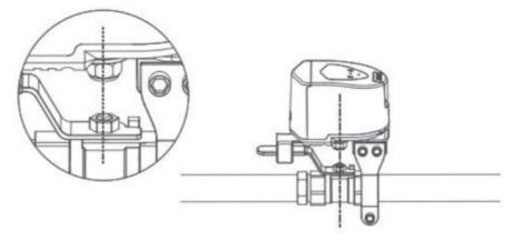
4. Tighten the mounting bracket screws to ensure the stability of the device.
