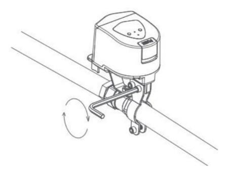
5. Open the battery compartment, install the batteries, and then re-close the battery compartment.
