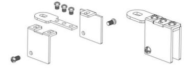
3. Use an Allen key or pliers to rotate counterclockwise, loosen the hex nut located below the device, and disassemble the nut, washer, and the swing arm for lever handles.
