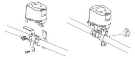
3. Move the device to the valve, secure the swivel arm to the valve handle, and take note of the mounting position of the controller, ensuring that the output shaft of the unit aligns with the center axis of the valve swivel.
