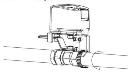
4. Move the device to the valve, attach the swivel arm to the valve handle, and carefully observe the installation
