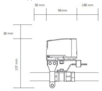
2. Pre-mount the 2 pieces of mounting bracket on the pipe using screws (do not tighten the screws yet).
