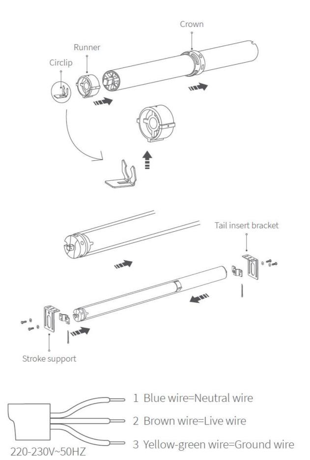
Put the motor into the wall of the shutter pipe and fix it firmly. Connect the control box to the RJ11 interface.
