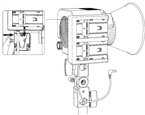
\*Batteries sold separately. Please press the seat button to remove the batteries. Do not pull it out forcibly.
