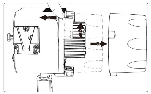
**Warning:** Always remove the protection cover prior to turning on the light. Always re-install the cover when packing it away.
