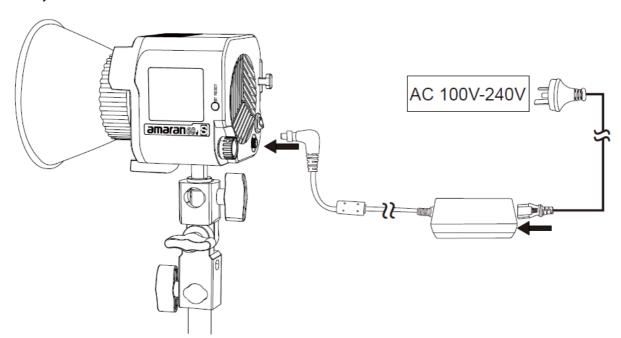
$^{\star}$ Please press the button on the DC interface to remove the power cord from the lamp.
