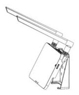
• Match the brackets lower buckle by gently press the lower side of the MACTM DTU until you hear a click. Please make sure the antennas are vertical to the wall.
