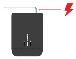
Connect reader to power supply. The center light will turn solid (not flashing) when ready.
