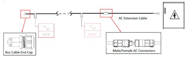
When AC extension cable is needed, users could connect the AC bus cable and AC extension cable in a junction box or use a pair of male/female AC connectors that APsystems provides as optional accessory.
