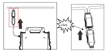
• Best Practice: Use the Bus Cable Unlock Tool of AC Bus to disconnect the connectors.
