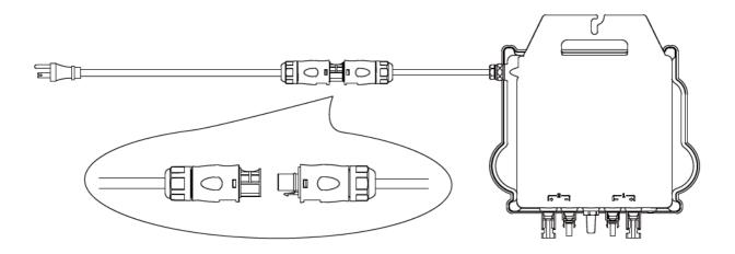
Insert the microinverter AC connector into the power cord connector.
