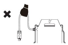
Do NOT carry the microinverter by the AC cable. This may cause the AC cable to partially or fully disconnect from the unit, resulting in no or poor operation.
