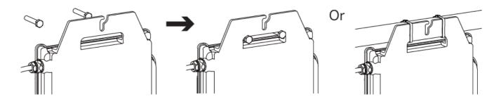
The Microinverter EZ1-LV can be installed on the balcony wall or fixed to the railing using cable ties. Select an appropriate installation method based on your actual scenario to ensure that the EZ1-LV is securely installed.
