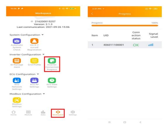
• The microinverters with "OK" are properly connected to the ECU.
