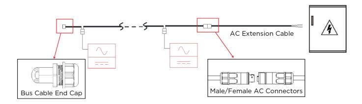
When AC extension cable is needed, users could connect the AC bus cable and AC extension cable in a junction box or use a pair of male/female AC connectors that APsystems provides as optional accessory.
