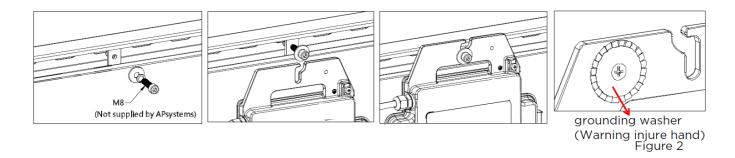
**WARNING:** Install the microinverters (including DC and AC connectors) under the PV modules to avoid direct exposure to rain, UV or other harmful weather events. Allow a minimum of 1.5 cm (3/4") below and above the casing of the microinverter to allow proper air flow. The racking must be properly grounded as per local electrical code.
