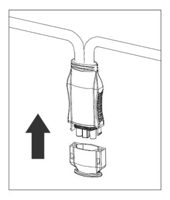
Step 6 – Install a Bus Cable End Cap at the end of AC bus cable
