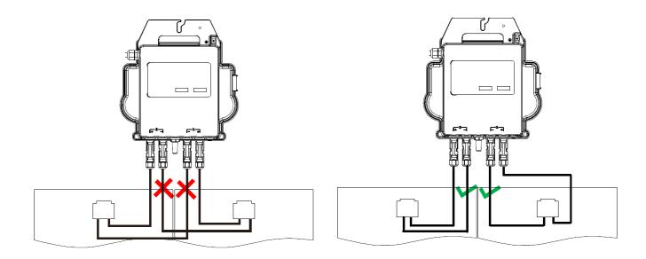
**WARNING:** Each PV panel must be carefully connected to the same channel. Make sure to not split positive and negative DC cables into two different input channels: microinverter will become damaged and warranty will not apply.
