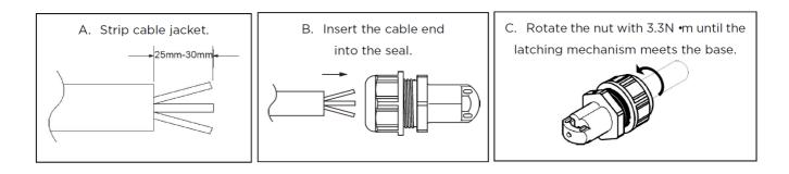
Step 7 – Connect APsystems Microinverters to the PV Modules
