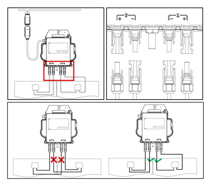
**Step 8. Connect APsystems Microinverters to Grid NOTE:**
