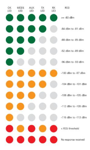
To enter Test Mode, press and hold the TEST button on the front panel until all the LEDs flash green (about 3-5 seconds).
