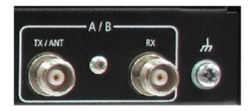
The antenna feeder cable should use grounding kits for lightning protection as specified or supplied by the coaxial cable manufacturer to properly ground or bond the cable outer.
