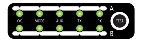
The Aprisa SR+ Protected Station has an LED Display panel that provides on-site alarms/diagnostics without the need for a PC.
