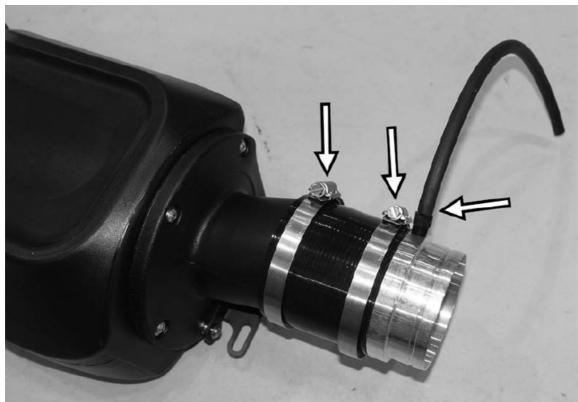
2. Attach the vacuum line to the vacuum fitting on the inlet adapter. Mount the inlet adapter to the back of either CI100035 or CI100039 with the silicone coupler and hose clamps supplied with the intake. Be sure to connect the vacuum line to the the car when mounting the intake assembly.
