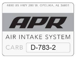
3. Once the APR intake is installed, be sure to clean a visible location under the hood and affix the supplied sticker in order to aid inspection of the vehicle under the California Smog Check program.
