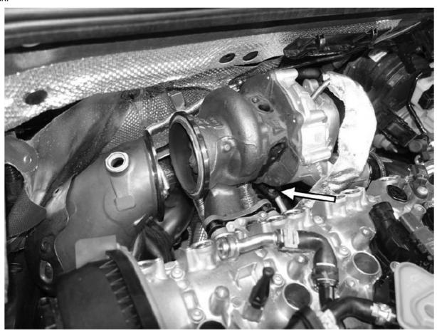
29. Carefully lift and rotate the turbocharger up and out of the engine bay, making sure not to snag or hit the turbo on anything while removing it.
