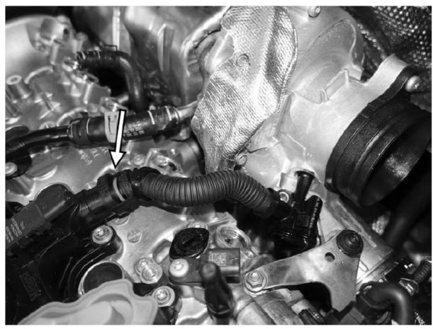
19. Remove the two T30 screws and one 10mm nut holding the turbo compressor support brace near the inlet of the turbo, and remove the brace from the car.
