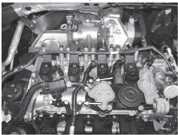
54. Lay the wiring harness back into its original location at the back of the engine. Reconnect the electrical connector to the high-pressure fuel pump and the turbo speed sensor on the back of the turbo (inset).
