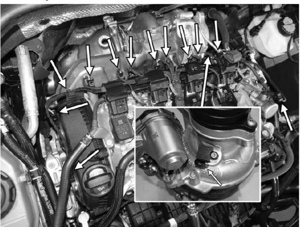
55. Secure the four ignition coil packs with the four original 10mm threaded studs. Tighten the studs to 9Nm (80 inlbs). Reconnect all four electrical connectors to the back of the coil packs.
