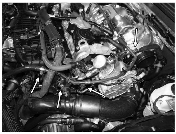
15. Remove the eight T25 screws from each of the valve lift solenoids.
