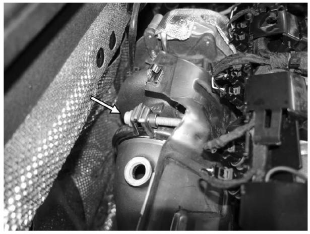
7. Remove the 13mm screw holding the downpipe bracket to the back of the engine block. As seen from below, this screw is just above the inner right CV axle joint. The down-pipe can now be separated at the turbocharger and moved to the right side of the engine bay.
