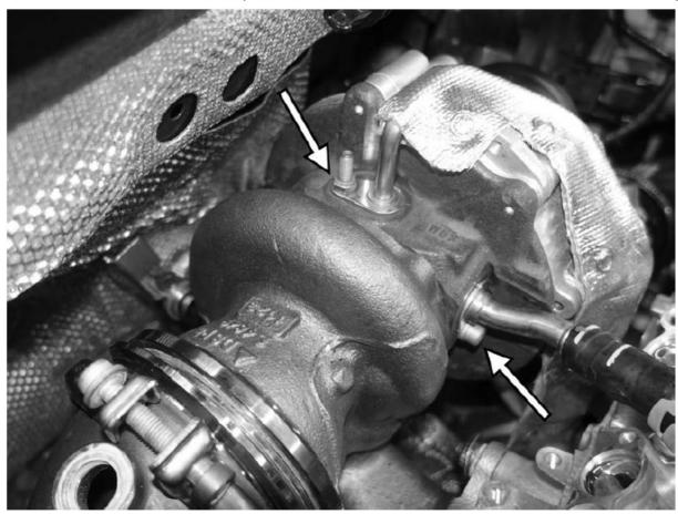
25. On the oil feed line, remove the 8mm triple square screw holding the feed line to the compressor side of the turbo. Separate the feed line from the turbo.
