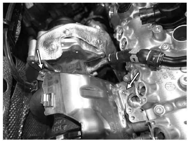
21. Remove the two 10mm nuts from the back side of the heat shield where the studs from the cylinder head mount the heat shield. Remove the heat shield from the car.
