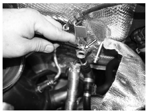
35. Remove the old turbo to the cylinder head gasket. Clean the mating surface of the cylinder head and then install the newly supplied gasket on the studs on the cylinder head.
