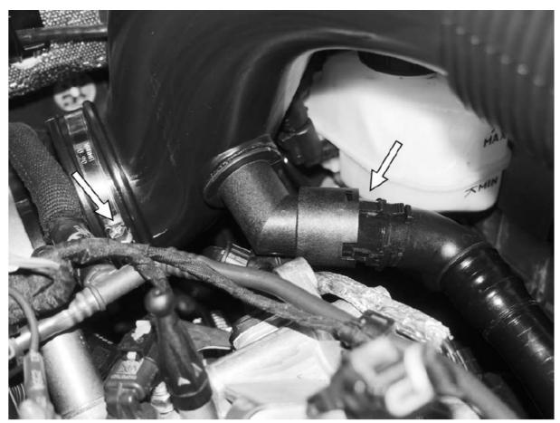
63. Reinstall the airbox assembly by first attaching it to the tabs on the back of the radiator core support, and then fully pushing it down on the three posts underneath. Rein-stall the two T25 screws on the front of the APR airbox and tighten them to 2Nm (18 in-lbs). Install the inlet pipe onto the back of the airbox, and tighten the 7mm nut on the clamp to 6Nm (53 in-lbs).
