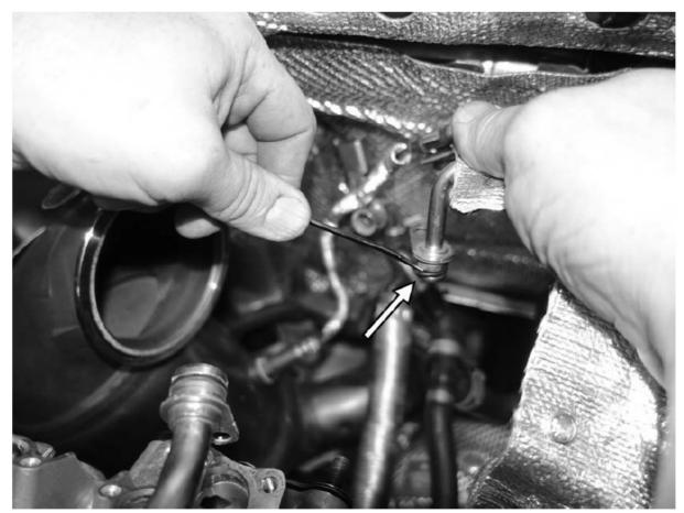
33. On the coolant return line still on the car, replace the o-ring with one of the supplied 15x2mm o-rings. There are two o-rings of this size supplied in the kit.
