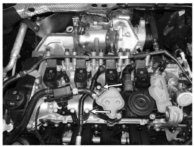
13. Disconnect the coolant line from the top of the coolant expansion tank. Remove the T30 screw holding the coolant line to the top of the valve cover. Disconnect the tee fitting on the coolant line behind the number two cylinder. Be careful not to deform the plastic coolant hose while working with it.
