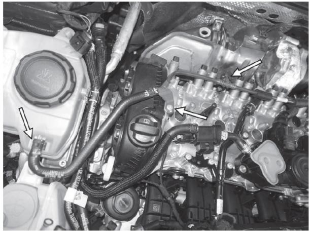
14. On the same coolant line, disconnect the two tee fittings behind the number four cylinder and one in front of the high-pressure fuel pump. Disconnect the hard coolant line from the coolant hose that runs by the factory airbox.
