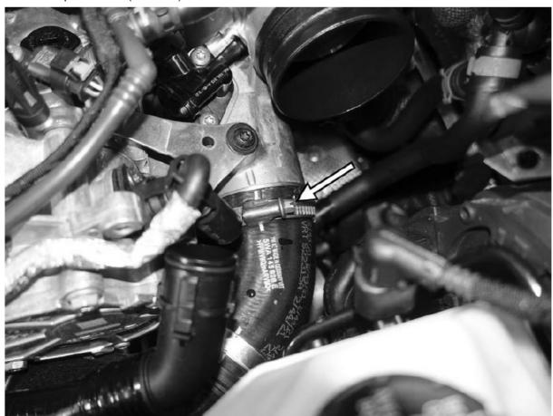
61. Reinstall the T30 screw holding the turbo outlet pipe to the side of the engine. Tighten the screw to 7Nm (62 inlbs). Reattach the wiring harness to the turbo outlet pipe.
