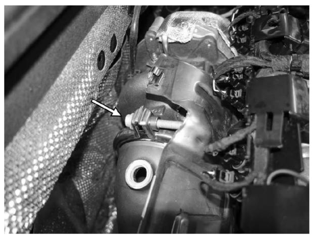
59. Reinstall the primary oxygen sensor into the stock downpipe with an oxygen sensor socket. Tighten the sensor to 60Nm (44 ft-lbs). Then route the harness for the sensor back to its original connection point, reclreclining harness into the mounting points. Reconnect the harness connector, and place it back into the bracket for the connector.
