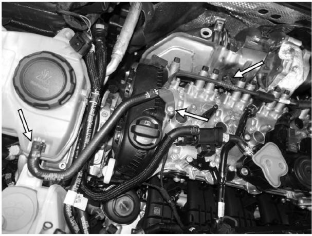
53. Reinstall the ignition coil packs in the engine, but do not secure them. Reinstall the two T30 screws holding the
