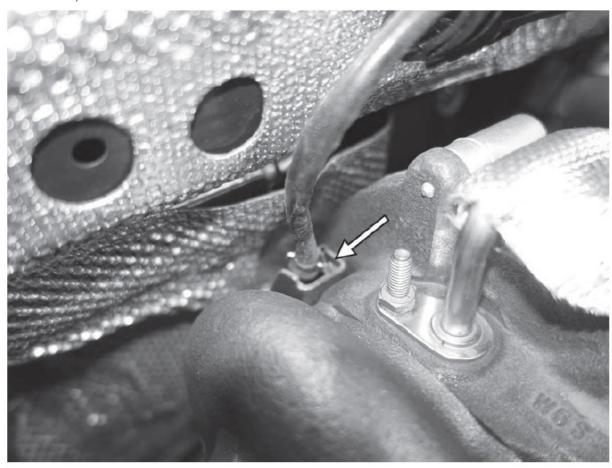
46. Reinstall the heat shield on the studs that protrude from the back of the cylinder head. Secure with the three 10mm nuts that originally held it in place and tighten the nuts to 8Nm (71 in-lbs).
