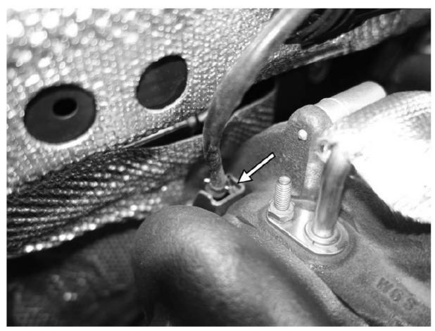
23. As pictured from behind the engine, follow the oil drain line from the bottom of the turbo down to where it connects to the engine block. Remove the 8mm triple square screw and separate the line from the engine block.
