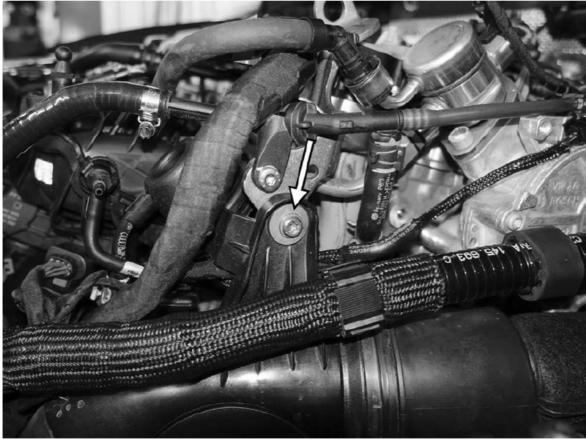
5. Disconnect the electrical connection for the primary oxygen sensor. Separate the connector from the bracket it is mounted in. Separate the harness from the two clips on top of the engine. Finally, using an oxygen sensor
