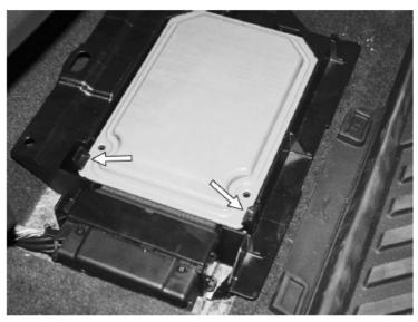
5. Pull on the tab on the electrical connector to the suspension con-troller, releasing the connector and remove the controller from the car.
