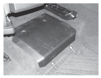
4. Push the plastic tabs on the right side of the suspension controller away from the controller, releasing it from the mounting bracket.
