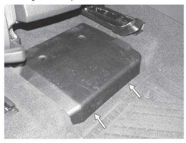
8. Reinstall the two push pin con-nectors holding the cover back to the floor.
