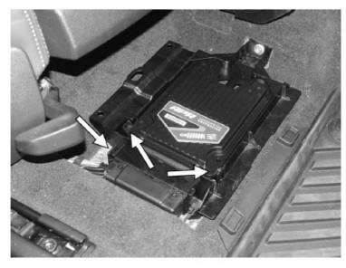
7. Slide the cover back over the electrical connector, ensuring the tabs on the back side of the front of the cover slide back in place on the mounting bracket. Replace the front floor mat if removed.
