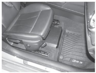
2. Remove the two push pin style clips from the cover under the front seat.
