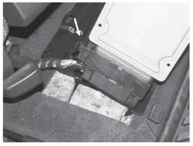
6. Connect the electrical connector on the APR suspension controller, and then place the controller into the mounting bracket on the floor. Make sure the two plastic tabs clip in place, securing the suspension controller.
