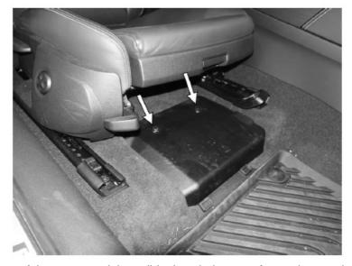
3. Slightly lift up on the front of the cover, and then slide the whole cover forward, towards the front of the car. It may be necessary to remove the front floor mat.
