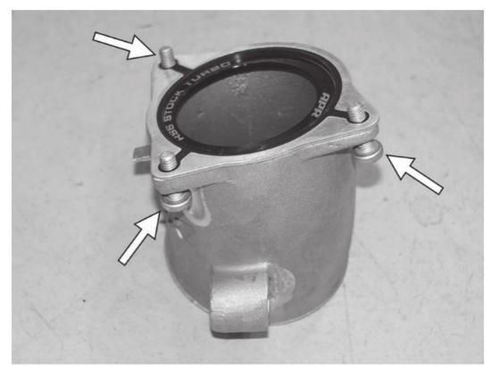
10. Install the APR cast turbo inlet pipes onto the front of the turbochargers with the six T30 screws. Start all six fasteners by hand, and then tighten and torque them to 9Nm (80in-lbs).
