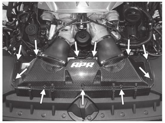
16. Adjust and tighten the clamps on the APR inlet hoses to the APR cast turbo inlet pipes. Torque the 7mm screws on the clamps to 7Nm(62in-lbs).
