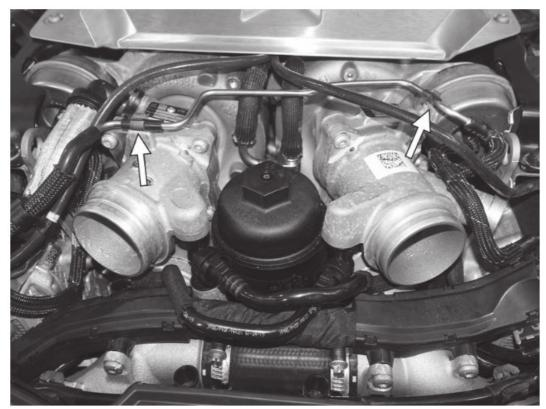
8. Remove the six T30 screws holding the OEM cast turbo inlets to the front of the turbos. Be careful not to drop the screws while removing them. Remove the cast turbo inlets from the car.
