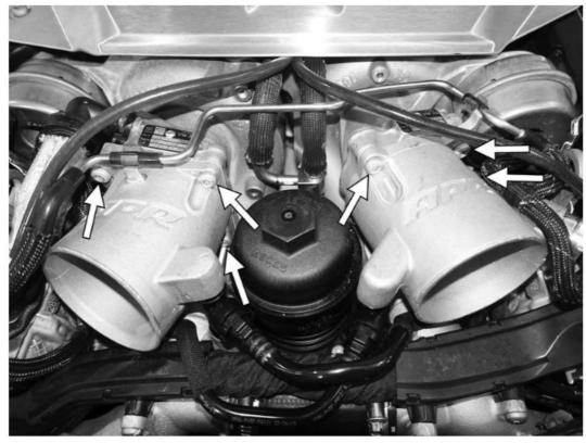
11. Reclip the hard vacuum lines onto the tabs on the top of the APR cast turbo inlet pipes.
