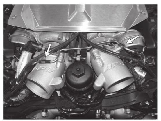
12. Install the ovalized APR inlet hoses onto the back side of the APR carbon fiber airbox cover. The flat side of the inlet hoses goes towards the bottom of the cover, and the raised hump side goes towards the top of the cover. Make sure the inlet hoses are fully seated on the cover. It is best to install the supplied clamps with the 7mm screws on the bottom side, so they will not be visible once installed. Tighten the 7mm screws on the clamps to 1.2Nm (10.5in-lbs).
