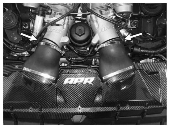
15. Secure the APR airbox lid by installing the eleven T25 screws and torquing them to 1Nm (9in-lbs).
