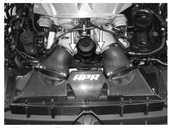
17. Reconnect the PCV valve to the right APR cast turbo inlet pipe by pressing it in place.
