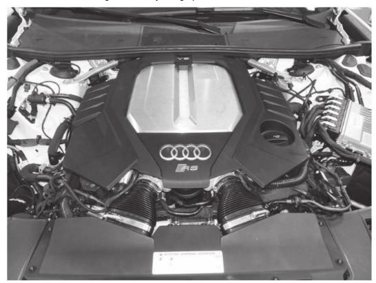
2. Remove the eleven T25 screws holding the top of the OEM airbox lid.
