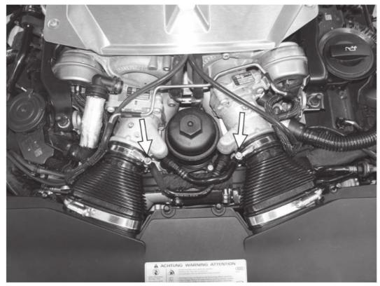
4. Left and remove the OEM airbox lid with the accordian hoses attached to expose the OEM air filter.
