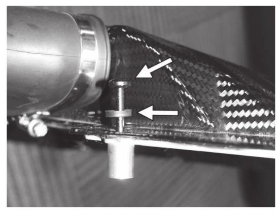
14. Place the APR airbox lid assembly onto the car, aligning the APR inlet hoses onto the APR cast turbo inlet pipes.
