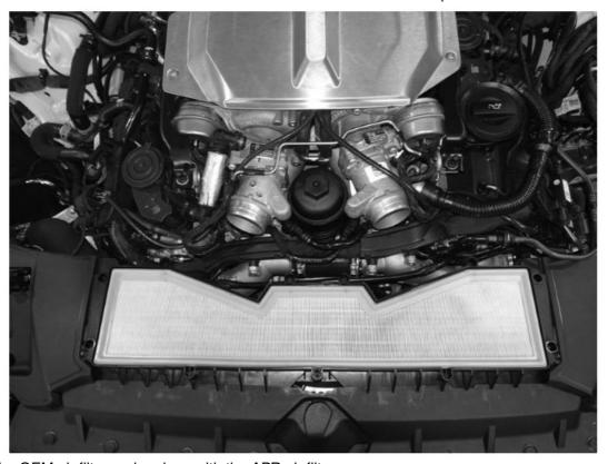
5. Remove the OEM air filter and replace with the APR air filter.
