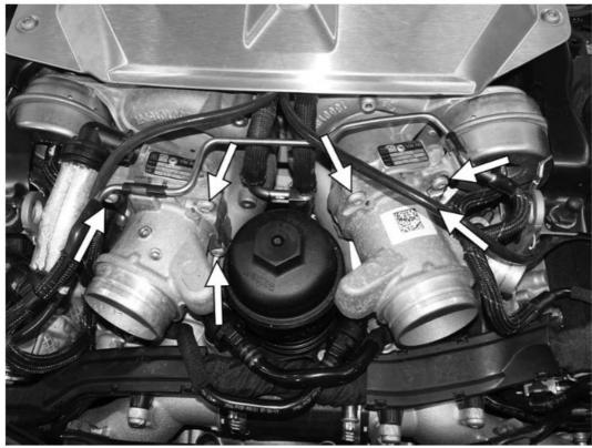
9. The inlet adapter ring for the stock turbos comes installed in the APR cast turbo inlet pipes. If using different turbos, uninstall the stock dapter rings and install the adapter ring for the turbos you are using. Place the supplied gasket on the inlet pipe flange, and loosely preinstall the six T30 screws through the casting and into the gasket. The gasket should retain the screws.
