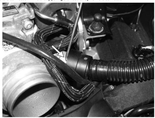
7. Unclip the hard vacuum lines from the top of the OEM cast turbo inlets.
