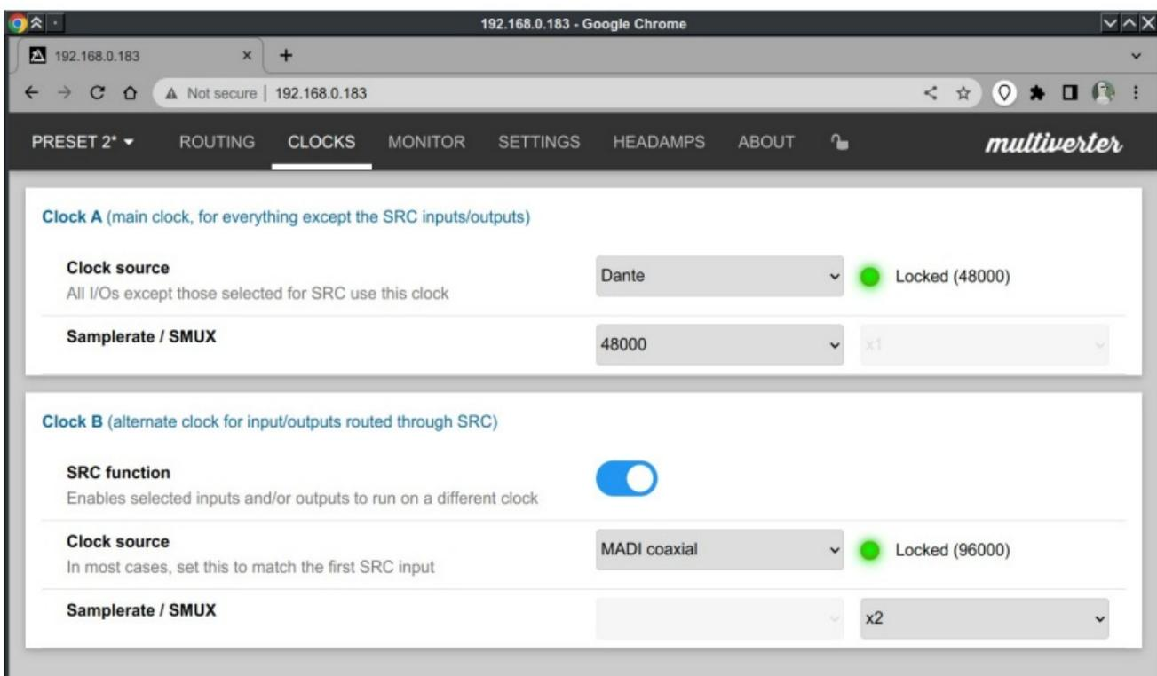
When the SRC module is installed and enabled, its behavior can be selected in the SRC section on the bottom. The settings above show a typical configuration for converting MADI 96k to Dante 48k.
