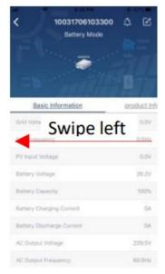
**Basic Information** displays basic information of the inverter, including AC voltage, AC frequency, PV input voltage, Battery voltage, Battery capacity, Charging current, Output voltage, Output frequency, Output apparent power, Output active power and Load percent. Please slide up to see more basic information.
