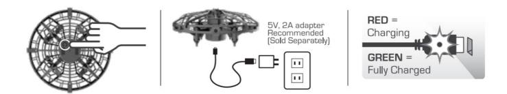
Plug included charging cable into drone and USB power supply.
