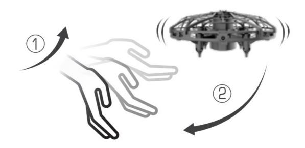
Turn drone on and hold it upright in front of you in the palm of your hand. Keep drone level and give it a slight toss upward, then drop your hand quickly downward.
