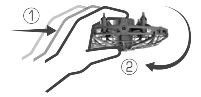
Quickly grab drone and flip upside down to stop. If out of reach, blast drone to make it fall or wait until battery power is depleted. Drone will auto-land itself.
