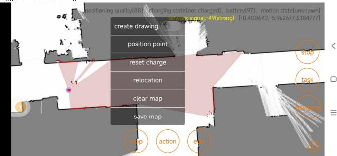
Control PPBot to the desired location for adding a point and rotate it to the specified angle.
