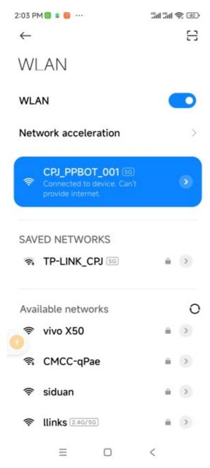
After completing the WLAN settings, open the mapping software and enter the IP address of PPBot. The default IP is 192.168.11.1. Click the "Connect" button.
