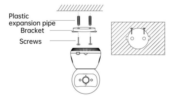
The dome camera can be installed on the wall or ceiling.
