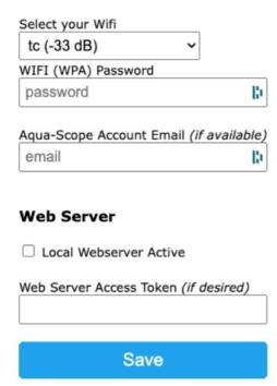
The device will act as open WIFI access point with the SSID 'Scope'. You need to connect your mobile device or PC to this SSID. Start a web browser and open the page: <a href="http://192.168.1.4">http://192.168.1.4</a>.
