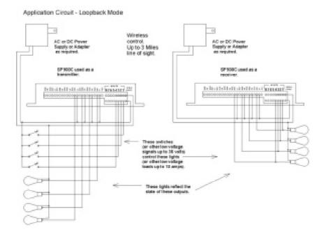
In loopback mode, the relay is activated as in the earlier example. However, in Loopback mode, a transmission will then be sent back to the originating location and a relay activated as feedback that the remote operation has been carried out.
