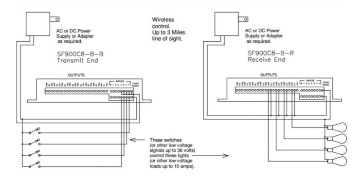
APPLIED WIRELESS SF900C Standard One Way Application 4 of 8 circuits shown
