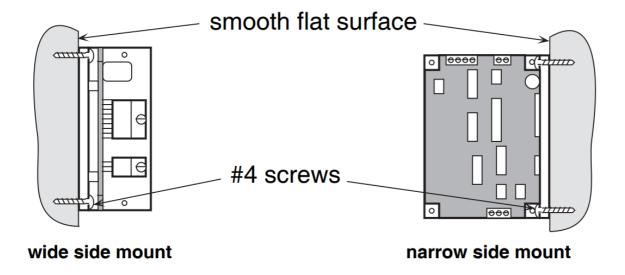
To operate the drive continuously at maximum power you must properly mount it on a heat sinking surface with a thermal constant of no more than 4°C/watt. Often, the metal enclosure of your system will make an effective heat sink.
