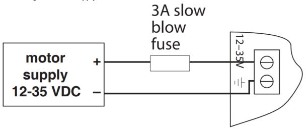
DO NOT REVERSE WIRES - THIS WILL DAMAGE THE DRIVE
