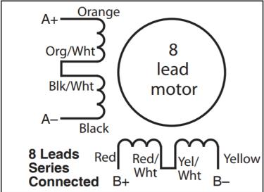
**Warning:** When connecting the motor to the driver, be sure that the motor power supply is off. Secure any unused motor leads so that they can't short to anything. **Never disconnect the motor while the drive is powered up. Never connect motor leads to ground or to a power supply!**
