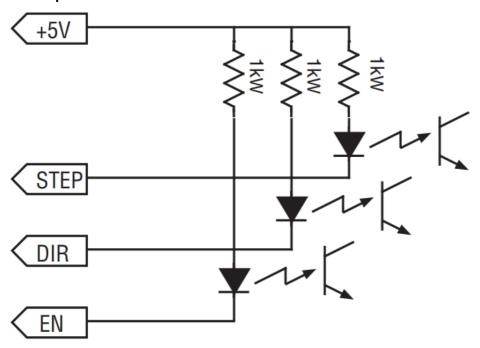
Your controlling logic must be capable of sinking at least 5 mA to control each drive input. Most CMOS and open collector TTL devices are directly compatible with this drive. Logic low, or 0, for a given input occurs when that input is pulled to less than 0.8 volts DC. In this state the LED is conducting current. Logic high, or 1, occurs when the input is greater then 4 volts or open.
