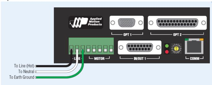
Wire the drive to the AC power source. (do not apply power until all connections to the drive have been made)
