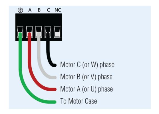
Connect the drive to the motor. If you are using one of the recomended Applied Motion motors, connect the motor as shown. Be sure to connect the motor case ground to the SVAC3 ground terminal. For a non-Applied Motion Products motor, please refer to your motor specs for wiring information.
