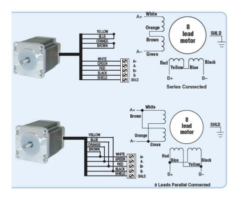
Wire the motor. See the STAC6 Hardware Manual for further details.
