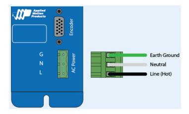
Wire the drive to the AC power source. (apply power only after step 4 is completed and the programming cable is connected)
