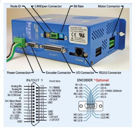
• Wire the drive to the AC power source. (Do not apply power until Step 3)
