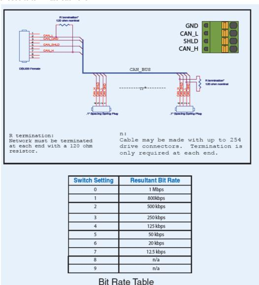
Set BitRate, Node IDCANOpen Bitrate – AMP CANOpen drives have three sets- things, one for Bit Rate and
