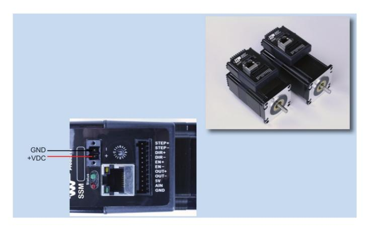
Note – the SSM drive accepts DC voltages from 12-70V. If using an external fuse, we recommend a 4 amp fast acting fuse .
