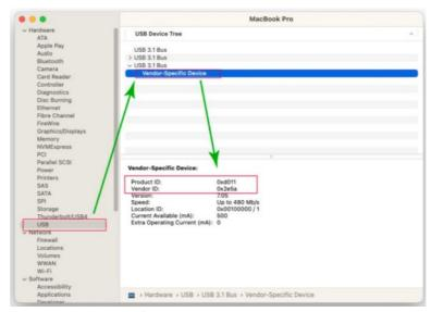
**NOTE:** If your Mac cannot find the 'Vendor-Specific Device with VID/PID 0xd011/0x2e5a for the VF3240 device, it means that the scanner is not recognized in your MacOS. To resolve this issue, try connecting the scanner
