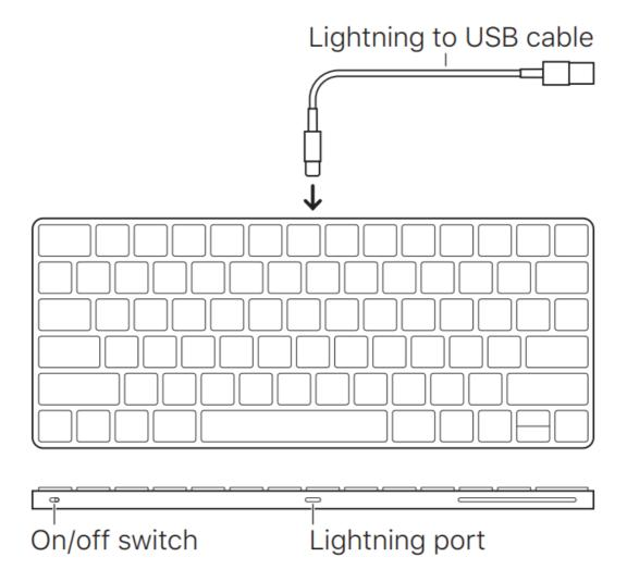
To pair your Magic Keyboard with your Mac, use the Lightning to USB cable that came with your keyboard. Plug the Lightning end into the Lightning port on your keyboard, and the USB end into a USB port on your Mac. Slide the keyboard on/off switch to on (so you see green on the switch).
