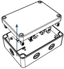
• Remove the appropriate knock-out on the underside or lower rear of the casing, install the M16/20 IP-rated gland.
