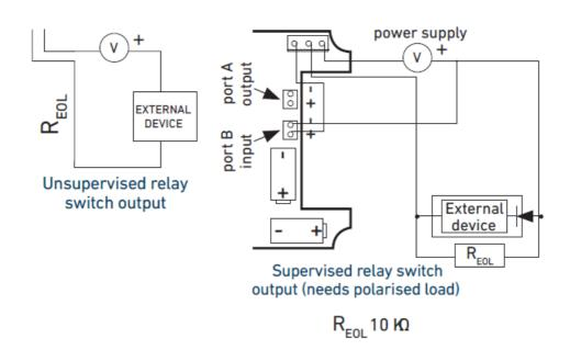
• Ensure the device connected to the unit is not drawing more than 2 A at 30V (no 220 VAC). Drawing too much current through the output relay or connecting mains voltage could possibly damage the unit and void the warranty.
