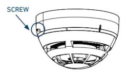
• Secure the screw on the base to ensure there is no unwanted removal using a M3 allen key.
