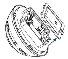
• Remove the battery compartment cover on the base on the detector.
