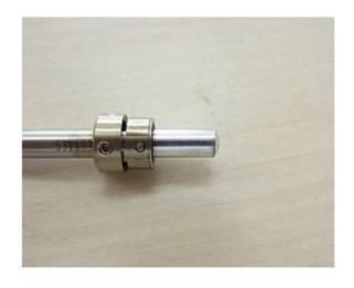
3. Wipe off the burning inhibitor substance stuck on the top of DX-HET. It can be easily wipped off with a dry cloth.
