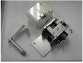
2. Loosen the set screw "1" for alignment cutting blade shaft and the setting nut "2" to adjust the shaft position. Then move the blade shaft position to match the center of the cutting blade and V grove of the lower roller.
