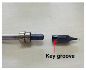
6. Make sure that burning inhibitor substance has been applied to the whole top of DX-HET as shown on the left. Then insert the X-tip firmly while adjusting the key groove to the correct position.
