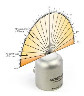
Directional, or cosine, the response is defined as the measurement error at a specific angle of radiation incidence. Error for Apogee SQ-600 series Extended Range PFD Sensor is approximately  $\pm$  2 % and  $\pm$  5 % at solar zenith angles of 45° and 75°, respectively.
