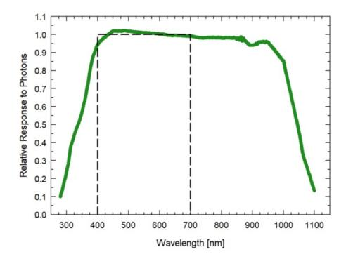
Mean spectral response measurements of six replicate Apogee SQ-600 series Extended Range PFD Sensors. Spectral response measurements were made at 10 nm increments across a wavelength range of 300 to 1100 nm in a monochromator with an attached electric light source. Measured spectral data from each PFD sensor were normalized by the measured spectral response of the monochromator/electric light combination, which was measured with a spectroradiometer
