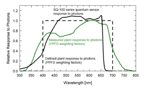
Defined plant response to photons (black line, weighting factors used to calculate PPFD), measured plant response to photons (green line, weighting factors used to calculate YPFD), and SQ-100 series and SQ-300 series quantum sensor response to photons (sensor spectral response).
