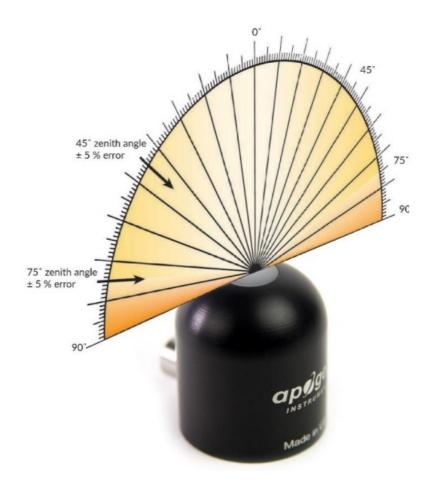
Mean cosine response of five SQ-100 series quantum sensors. Cosine response measurements were made by direct side-by-side comparison to the mean of seven reference SQ-500 quantum sensors from the mean of replicate reference quantum sensors (LI-COR models LI-190 and LI-190R, Kipp & Zonen model PQS 1). Data were also collected in the laboratory using a reference lamp and positioning the sensor at varying angles.
