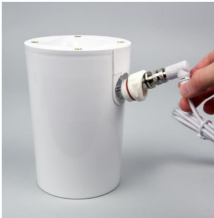
Push the EE08 into adapter port.
