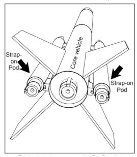
This basic design was created by Ray Dunakin in the 1990's. It was featured in the 2008 book Model Rocket Design and Construction by Tim Van Milligan. What we changed in the design is the shape and size of the attachment hooks to make the rocket more aerodynamic, so that it can fly even higher in the sky. We also laser cut the wood parts to make assembly more precise so that everything fits nicer and goes together easier.
