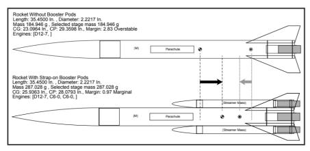
The strap-on pods will move the CG rearward, and the CP forward on the rocket. Make sure the CG remains ahead of the CP position.
