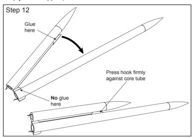
step 10. Rotate the strap-on pod toward the tube so that the forward hook touches the core tube. Make sure the pod is straight along the tube before you press it into place. Allow the glue time to harden before removing the nose cone and taking off the pod.
