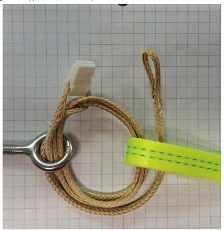
• Step 4: Route the looped end through the opening on the stopper end, and then route the stopper through the loop.
