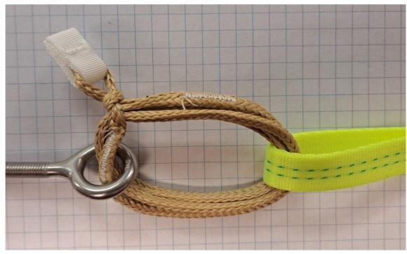
The number of wraps or passes through all items will dictate the break strength rating of the soft link. It is recommended that the working load not exceed 20% of the break strength.
