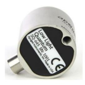
A sensor's model number and serial number are located on the bottom of the sensor. If the manufacturing date of a specific sensor is required, please contact Apogee Instruments with the serial number of the sensor.
