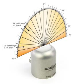
Mount the sensor to a solid surface with the nylon mounting screw provided. To accurately measure photon flux density incident on a horizontal surface, the sensor must be level. An Apogee Instruments model AL-100 leveling plate is recommended for this purpose. To facilitate mounting on a cross arm, an Apogee Instruments model AL-120 mounting bracket is recommended.
